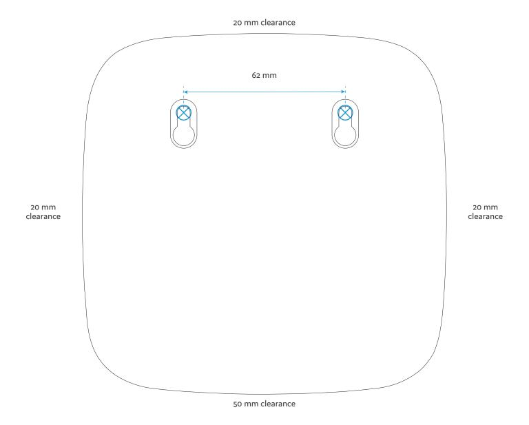
$igorplus ext{Drill bit } \emptyset ext{ 6 mm} ext{Unit mm}$  Hole depth 35 mm ext{Scale 1:1}
